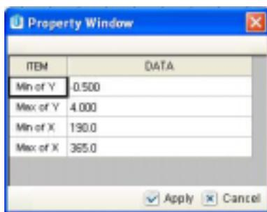
Set minimum/maximum wavelength (y-axis) and absorbance or transmittance (x-axis).
